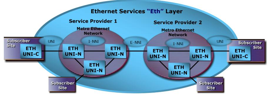
UNI: User Network Interface, UNI-C: UNI-customer side, UNI-N network side NNI: Network to Network Interface, E-NNI: External NNI; I-NNI Internal NNI
